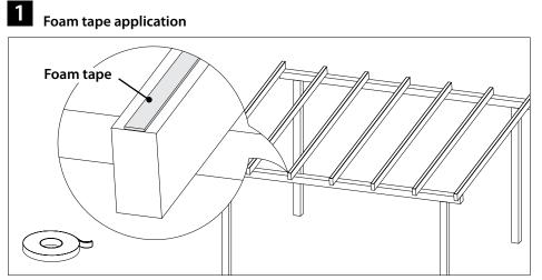
Applying foamed tape on each rafter will reduce friction.
