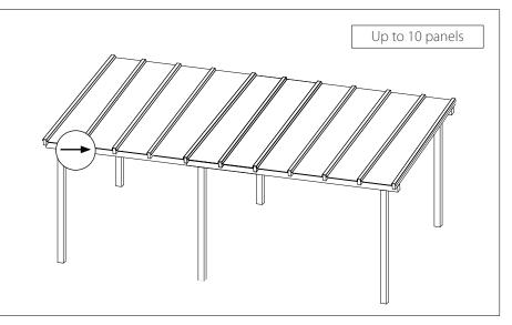
For 10 panels or less, start on one end of the structure and work across.
