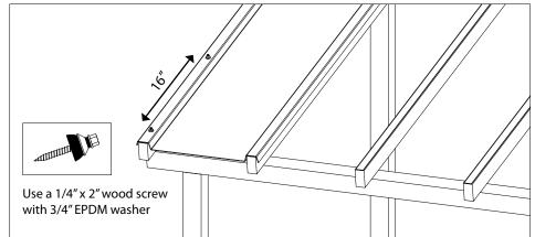
Attach the first EZ Glaze panel's outer corrugation, using specified screws and washers through the pre-drilled holes. Start at the bottom edge and work your way up.
