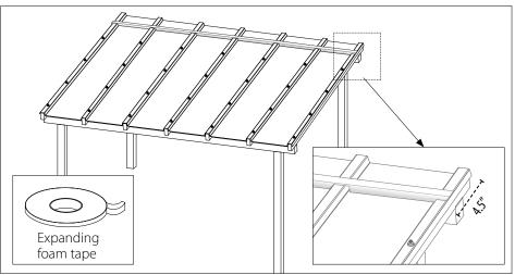
Expanding foam tape must expand to a dimension no less than 1.75".
