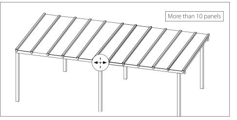
For more than 10 panels, start in the center of the structure and work out in both directions.
