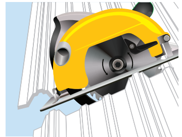
Sawing the panels Figure 4
